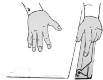
1. Open the clamping top bar by pulling the the flat front piece up and away from the back piece. This opens a slot along the bottom.
