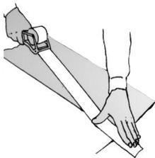
4. IMPORTANT: Reinforce the included Adhesive Strip by using a 2" packing tape, half on the print and half on the Leader.
